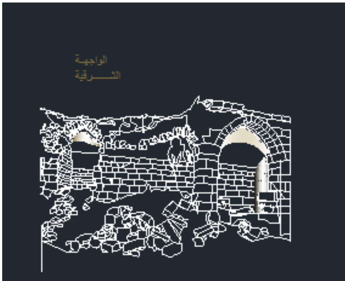
East side façade and gallery showing damage from 2015 airstrike
